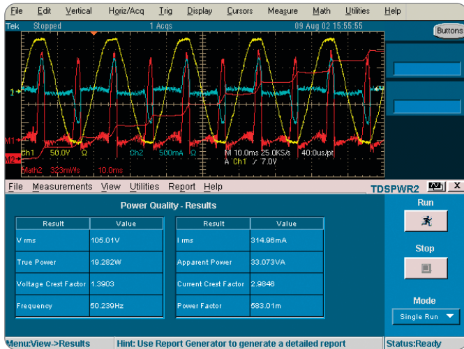
► Figure 4. Power quality measurements using TDS5000/7000 Series.
